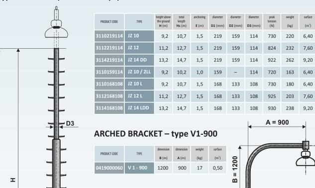
Steel poles type JZ and JZL for Czech Railways are equipped with brackets V1–900 and with special lighting. Lights are controlled with the lifting device situated in the shaft of the pole. mainpulation of the the lights is done using the handle.
